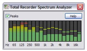
2. Optionally, select the "Peaks" check box to display peak levels for the individual frequency bands.
